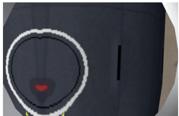
SRV on final approach. Real-time feedback of position, speed, heading and flight dynamics helps pilot align with hatch
