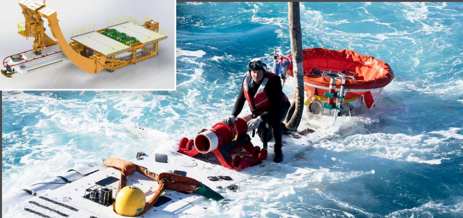
The 3rd generation system has a compact architecture and design. The system can be deployed in multiple layouts; meaning it can also be installed on vessels with unusual deck arrangements. The system is modular and various aspects can be deployed independently – for example individual Deck Decompression Chambers (DDCs) can be deployed independent of the rest of the system for escape support or secondary roles.
