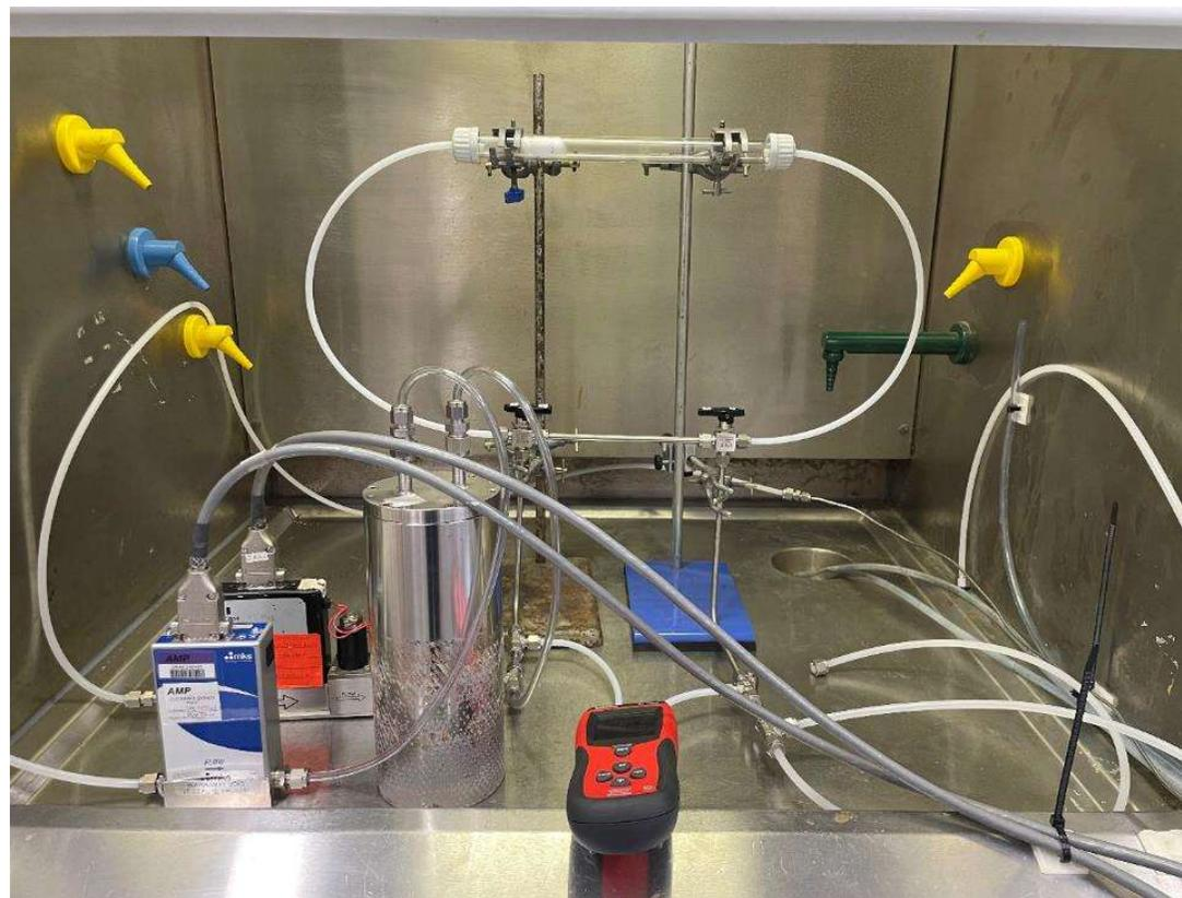
Figure 4: Experimental apparatus for  $\text{NH}_3$  tests
