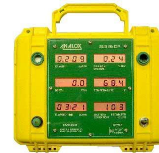
Analox and Anagas hyperbaric O 2 and CO 2 monitors (1990s)
