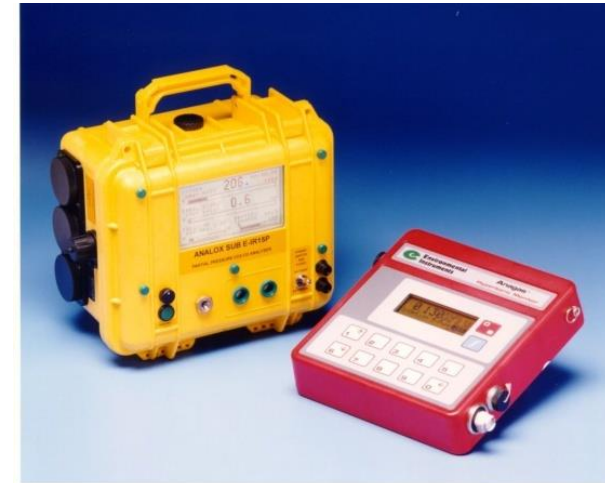
Analox and Anagas hyperbaric O 2 and CO 2 monitors (1990s)
