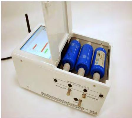
**Replaceable sieve packs are the only maintenance required (~ 6 months)**
