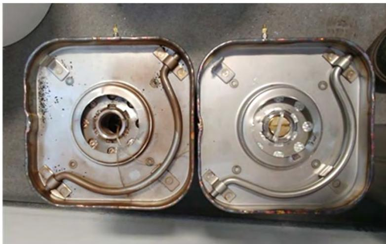
Difference between MPOG with a brass plug and without after opening pressurised units
