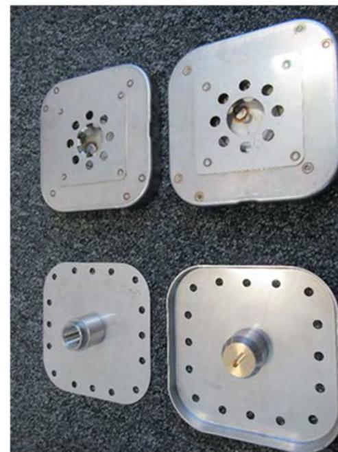
Shows the filter plate and underside of the lid of both the new including brass plug (right) and old design (left)
