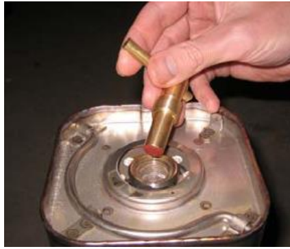
Fig 4. The Phosphorous tipped match for igniting the MILSPEC MPOG
