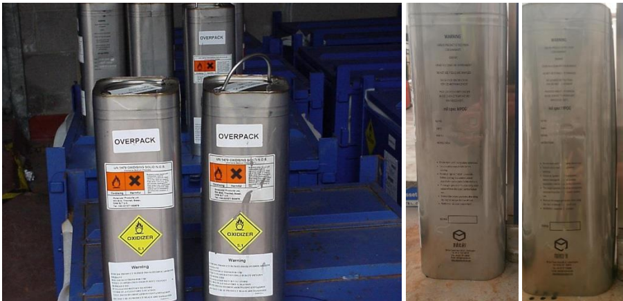
Figs.5-7 Swollen MILSPEC MPOG(right) in Faslane Stores next to standard MILSPEC MPOG and comparison next to straight edge in the laboratory.
