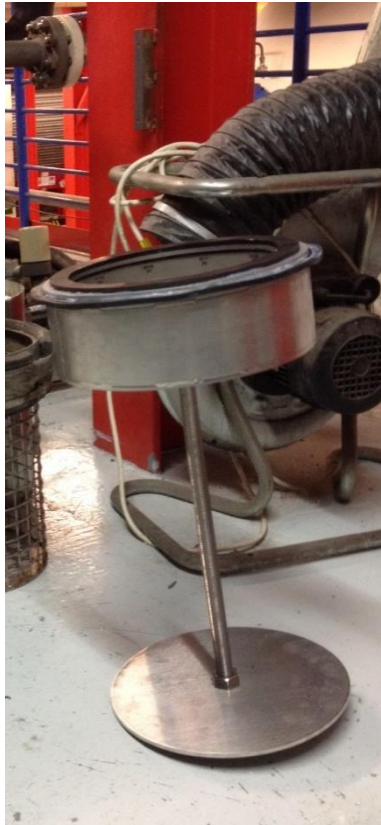
Base height adapter and seal; placed ExtendAir assembly in proper flow position
